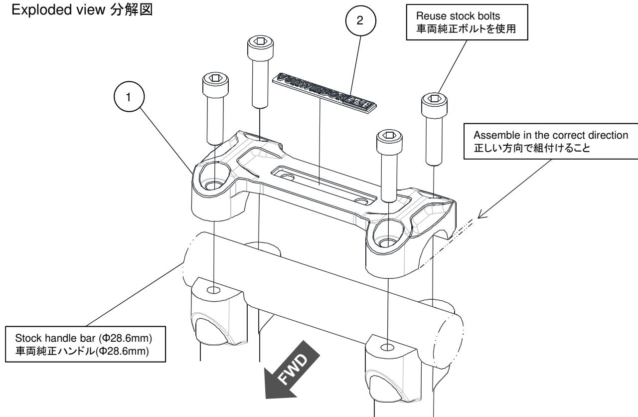
1. Replace the handle clamp following the correct procedure and tightening torque as specified in the genuine service manual.
