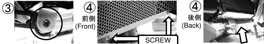
**CAUTION** Make sure that there is proper clearance between radiator core and protector. It is recommended to put sponge tape or rubber sheet at mounting bracket or at frame area to make a clearance.
