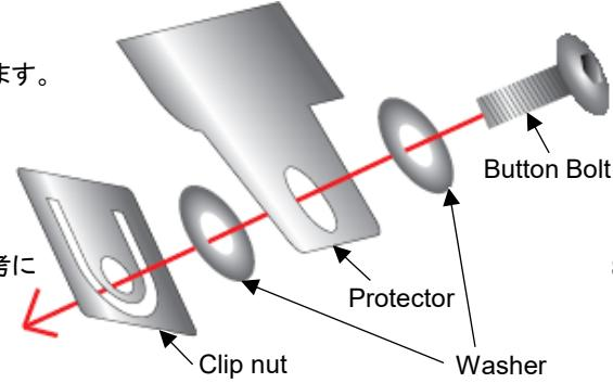
**CAUTION** Make sure that there is proper clearance between radiator core and protector. It is recommended to put sponge tape or rubber sheet at mounting bracket or at frame area to make a clearance.
