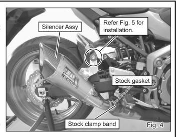
Check that there are proper clearances between Yoshimura slip-on and other components. Then, tighten and torque Button Bolt M6x20 and Cap Bolt M10x65P1.25 on Silencer Bracket, stock clamp band in order (See Fig. 6 & 7).
