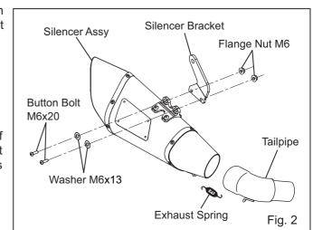
5) Install Silencer Assy to Tailpipe and fix them with Exhaust Spring (See Fig. 2).
