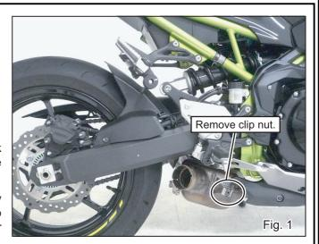
3) Remove clip nut from stock chamber (See Fig. 1).
