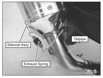
8) Install 2 of Exhaust Springs on each spring hook. (See Fig. 6)
