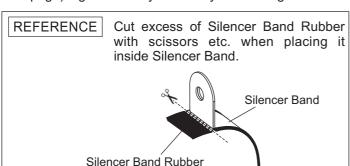
**CAUTION** Be sure to place Silencer Band at right angles to Silencer Assy. If neglected, it may cause breakage to Silencer Band.
