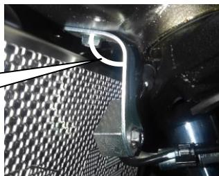
CAUTION! : Make sure that there is proper clearance between radiator/oil cooler core and protector.
