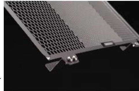
**CAUTION** Make sure that there is proper clearance between radiator core and protector. It is recommended to put sponge tape or rubber sheet at mounting bracket or at frame area to make a clearance.
