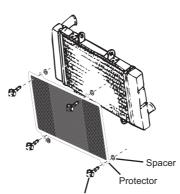
CAUTION!: Make sure that there is proper clearance between radiator/oil cooler core and protector. If neglected it may cause a damage of core, and it is recommended to put sponge tape or rubber sheet at mounting bracket or at frame area to make a clearance.
